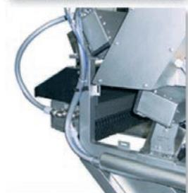
upper part, and double vision systems that inspect the product on both the upper and lower part. Each vision unit is equipped with a brush cleaning system for the periodic cleaning of the optical sections.
